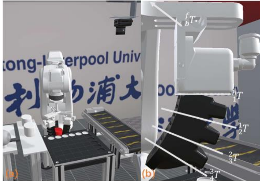
Fig. 4: Four Piecewise Robot Independent Mapping Soft Gripper: (a): Flexible gripper with robot working screenshot (b): Assembled Together Four-piece Soft gripper constant curvature model with four homogeneous transformation matrix T in Unity 3D; (c): Arc Configuration Space for only One piece soft gripper when angle \phi rotates the arc to new x' axis.
